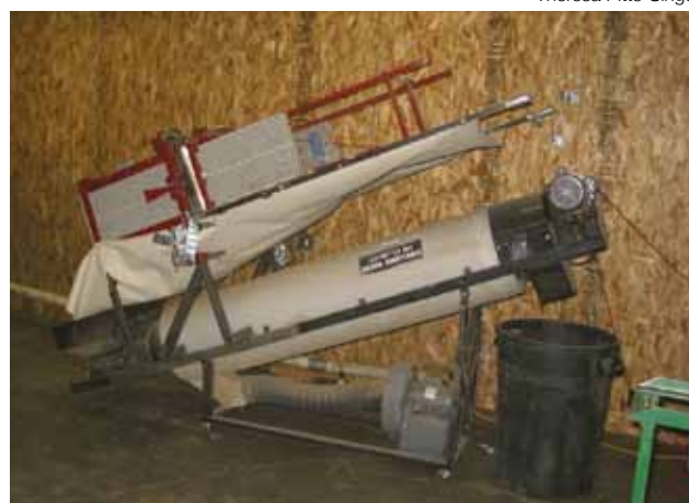
Figure 7.19 Automated cell harvesters use a series of plunger rods to punch out bee cells from Styrofoam nest blocks into a collection unit below. This particular model incorporates cell tumbling and separates excess leaf litter from the cocoons which are ejected into the garbage can at the right.
