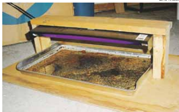
Figure 7.21 A homemade light trap to control chalcid wasps. The trap consists of a black light suspended over a pan of water containing a few drops of detergent to reduce surface tension. Light traps should be maintained in incubators and anywhere dormant leafcutter or mason bees are stored. Note the large numbers of drowned wasps in the pan.
